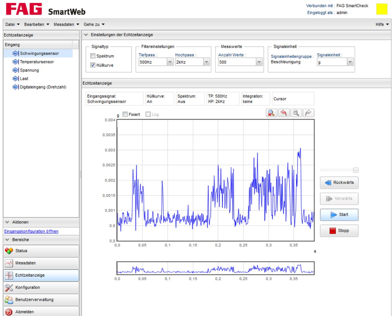
The screenshot shows the FAG SmartWeb interface. At the top left is the FAG SmartWeb logo. On the top right, it says 'Verbunden mit: FAG SmartCheck' and 'Eingeloggt als: admin'. Below this is a navigation bar with 'Datei', 'Bearbeiten', 'Messdaten', 'Gehe zu', and 'Hilfe'. The main interface is divided into several sections:
